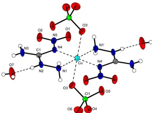
**Figure 3.** Molecular moiety of 5. Thermal displacements of non-hydrogen atoms were set at 50% probability. Hydrogen atoms are shown as spheres of arbitrary radius. Selected coordination distances (Å): Cu–N1 1.982(2), Cu–N4 2.032(2), Cu–O3 2.4364(19), angles (deg): N1–Cu–N4 79.58(9), N1–Cu–O3 85.41(10), N4–Cu–O3 83.44(8). Symmetry codes: (i)  $-x, 1-y, -z$ .
