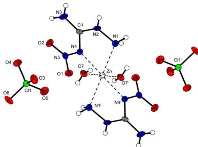
**Figure 4.** Molecular moiety of 6. Thermal displacements of non-hydrogen atoms were set at 50% probability. Hydrogen atoms are shown as spheres of arbitrary radius. Selected coordination distances (Å): Zn–N4 2.106(2), Zn–N1 2.148(2), Zn–O7 2.164(2); angles (deg): N4–Zn–N1 74.70(8), N4–Zn–O7 88.51(8), N1–Zn–O7 84.43(10). Symmetry codes: (i)  $-x, 1-y, -z$ .
