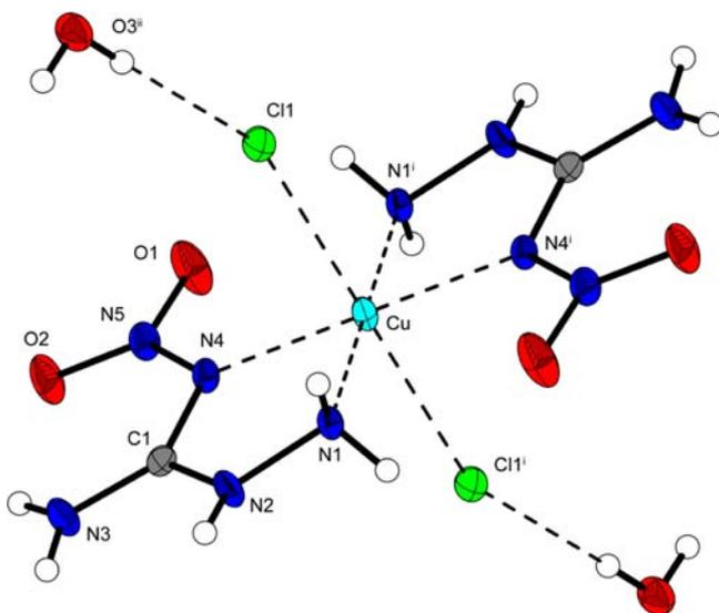
**Figure 13.** Molecular moiety of **18**. Thermal displacements of non-hydrogen atoms were set at 50% probability. Hydrogen atoms are shown as spheres of arbitrary radius. Selected coordination distances (Å): Cu–N1 1.997(2), Cu–N4 2.053(2), Cu–Cl 2.7155(7); angles (deg): N1–Cu–N4 79.14(8), N1–Cu–Cl 89.11(7), N4–Cu–Cl 89.90(6); Symmetry codes: (i)  $-x, -y, 2 - z$ ; (ii)  $-x, -0.5 + y, 0.5 - z$ .
